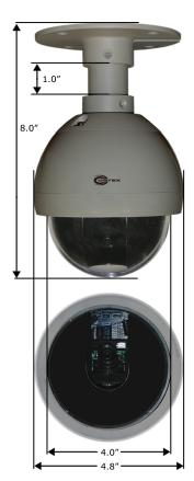
A single adapter cable connects to the dome for control signals, power, and video signals. An internal DIP switch determines communication protocol and dome addresses, which range from 0 to 255, allowing you to connect and address mutliple domes from a single controller.
