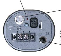
BNC VIDEO CONNECTOR PROVIDES COMPOSITE VIDEO OUTPUT AT 1Vp-p LEVEL (NOMINAL), 75 ohm impedance
