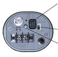
AUTO-IRIS CONTROL CONNECTOR MANUAL SWITCH FOR SELECTING BACK LIGHT COMPENSATION OR TURNING OFF COMPENSATION EN-TIRELY. USEFUL IN CERTAIN LIGHT/ ENVIRONMENTAL CONDITIONS
