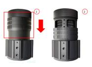
The varifocal lens has the normal manual adjustments for focus that you would find on any varifocal lens. To make adjustments, unscrew the knurled barrel cover and slide back, as shown in figure 1. This will expose the internal adjustment rings, as shown in figure 2. Adjust the lens using the inner knurled
