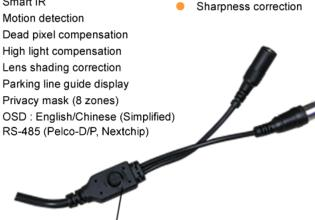
The 3-dimensional mini-joystick on the video/power cable gives the user quick access to the OSD menu. Move it left/right, up/down and "click" to navigate the menu and make selections
